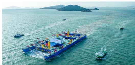
世界首艘自航式沉管运输安装一体船——“一航津安 1” The First Self-propelled Integrated Ship of Transportation and Installation of the Immersed Tubes in the World — "Yihang Jinan 1"
