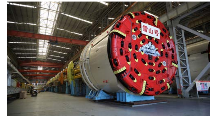
中交天和研发生产的“雪山号”盾构机用于天山胜利隧道施工 The "Xueshan" shield tunneling machine researched and developed by Tianhe is applied in the Construction of Tianshan Shengli Tunnel
